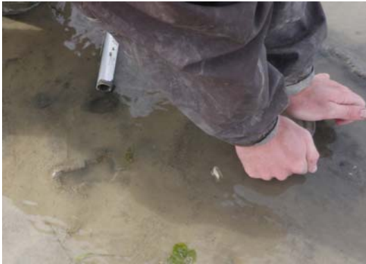
Figure 6. Sediment Grain Size Sampling Method Using a Core Sampler
