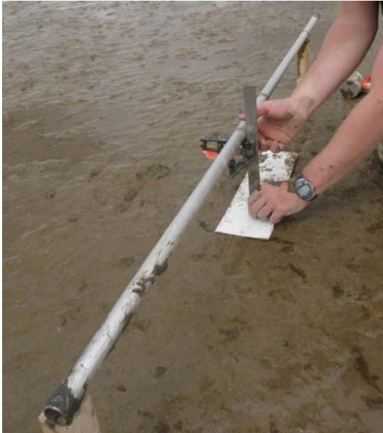
Figure 5. Accretion/Erosion Measurements Using the Sliding Ruler Placed at the Bottom of the Pole and to the Plastic Sheet on Mud
