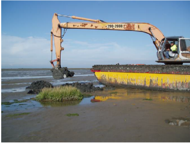
Figure 14. 2010 Linkbelt Amphibious Excavator Removing Spartina anglica at Brunswick Point, B.C.
