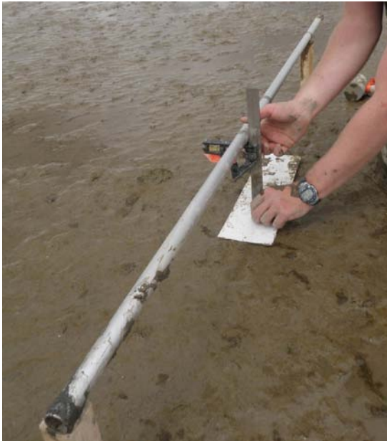
Figure 5. Accretion/Erosion Measurements Using the Sliding Ruler Placed at the Bottom of the Pole and to the Plastic Sheet on Mud
