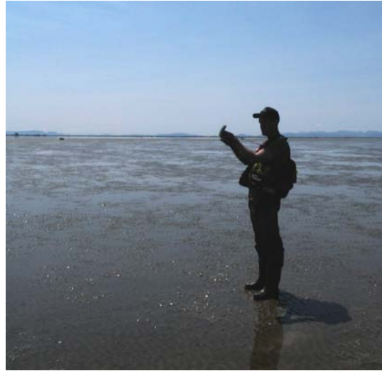
Figure 2. Transect Orientation Using a Compass
