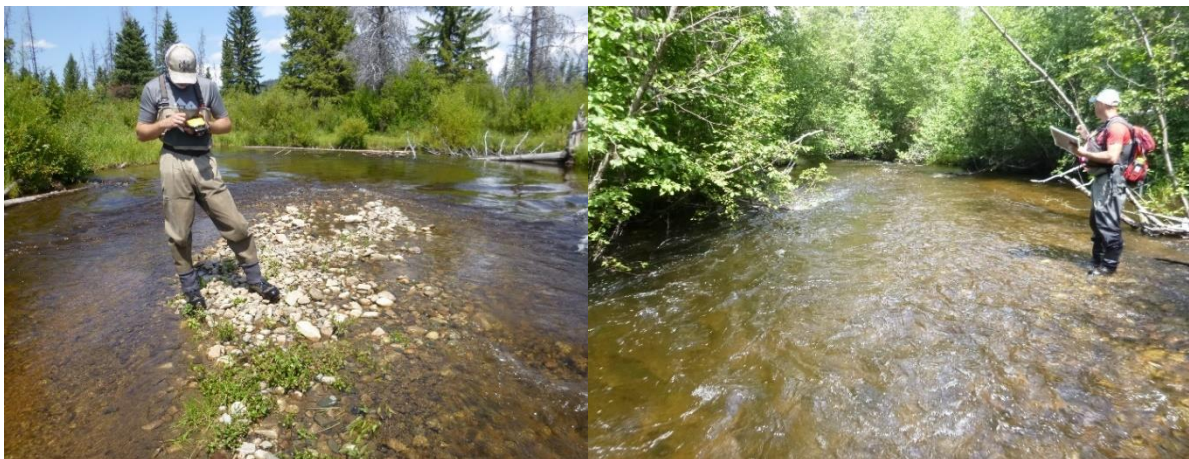
Entering data into the Trimble Geo 7x (Left) using the data dictionary developed specifically for RIM (Appendix D). Marking up large format field maps for subsequent incorporation into GIS mapping and integration into the final data deliverables (Right).
